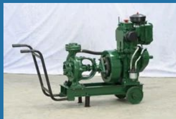
Diesel Pump Set
